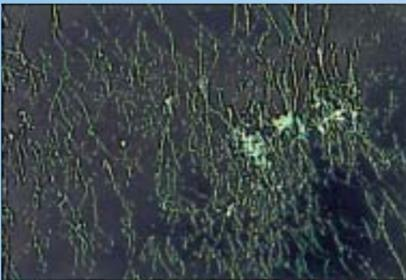
In regions where heat and humidity are high, mold is a constant threat. If you do not store your microscope in a cool, dry place, mold can grow on the lens surfaces, obscuring the images seen through the optical system. With the YS100, there is no need to worry. Thanks to Nikon's anti-mold paint and tablets, this is no longer a problem. In laboratory tests, mold did not form for up to five years, even at a 30°C temperature and 80% humidity.
