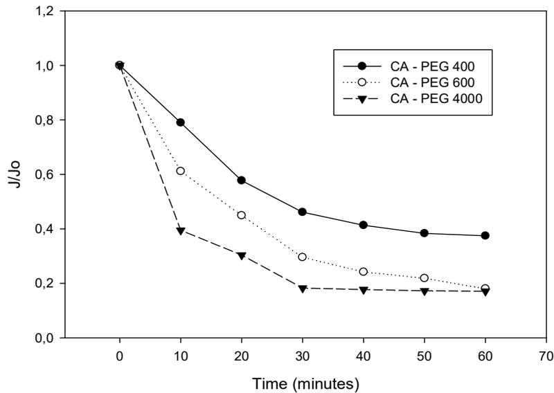
Fig. 7: Flux of the membrane during microfiltration.
