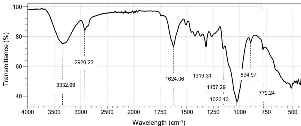
Fig. 2: FTIR spectra of cassava peel cellulose.
