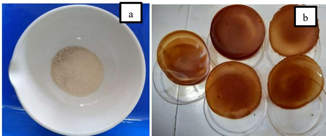
Fig. 4: (a) Cellulose acetate obtained from cassava peel cellulose; (b) CA-PEG membrane.
