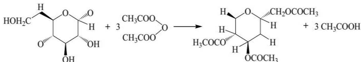
Fig. 3: The reaction of acetylation of cellulose.
